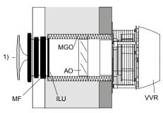
Mounting solution 2 If the MGO is shorter than the thickness of the wall, an inlet (ILU) and sleeve (MF) or spiral pipe (SR) must be installed, to which the diffuser (1) is attached.
