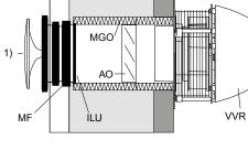
Mounting solution 2 If the MGO is shorter than the thickness of the wall, an inlet (ILU) and sleeve (MF) or spiral pipe (SR) must be installed, to which the diffuser (1) is attached.
