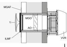
INSTALLATION SOLUTION 1 If a wall duct (MGO) terminates flush with the internal wall, a covering flange (MGAF) and inlet sleeve (ILMF) must be fitted before the diffusor is fitted (1).
