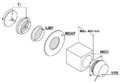
To ease installation an MGO wall duct can be used with the VVR wall fan.
