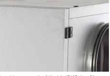
The cabinets are made of Aluzink AZ185 class C4 according to EN/ISO 12 944-2 and insulated with 50 mm mineral wool. This results in a low noise level to the surroundings/installation room.
