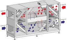
During wintertime operation with heat recovery, extract air enters at the top and is lead vertically down through the counterflow heat exchanger with any condensed water. The outdoor air enters from the bottom and runs up through the heat exchanger – i.e. a counter flow.
