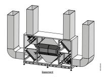
Included as standard is a mounting base with feet, which has an adjustable height of 130 - 160 mm.
