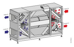
The design of the units means that in transitional periods and during summer, air can be led around the heat exchanger, via the bypass when their is reduces demand or no demand for heat recovery. The unit has a bypass on both the extract air and supply air side. Extract air and outdoor air is filtered during summer and winter operation and winter operation.
