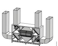
Included as standard is a mounting base with feet, which has an adjustable height of 130 - 160 mm.
