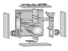
With some projects, limited space means that internal transport of the air handling unit is difficult or impossible. This is why the VEX300T is available as a SPLIT version. It means that the air handling unit can be assembled and tested at the factory as normal – just without sealant. The air handling unit can therefore be easily taken apart at the installation site, transported as single sections, assembled, sealed and commissioned. commissioned.
