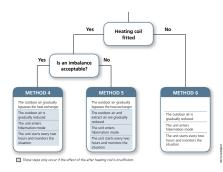
The control system monitors the actual airflow and also the pressure drop across the heat exchanger. If ice forms in the heat exchanger, the pressure drop across the heat exchanger will increase and when it exceeds a pre-set value, de-icing begins.
