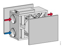
The side panels on both sides of VEX330H models can be removed (easy access). This allows the unit to function as both a LEFT and RIGHT version.
