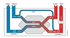
The VEX300T is designed with de-icing bypass. If there
