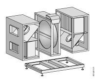
With some projects, limited space means that internal transport of the air handling unit is difficult or impossible. This is why the VEX200 is available as a split version. It means that the air handling unit can be assembled and tested at the factory as normal – just without sealant. The air handling unit can therefore be easily taken apart at the installation site, transported as single sections, assembled, sealed and commissioned.
