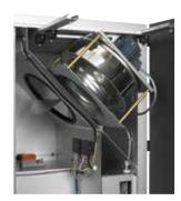
The motor sections are mounted in vibration dampers, which reduces noise in the ducts and eliminates the need to fit flexible connections between the unit and the duct system.
