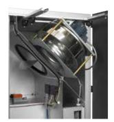
The motor sections are mounted in vibration dampers, which reduces noise in the ducts and eliminates the need to fit flexible connections between the unit and the duct system.
