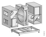
With some projects, limited space means that internal transport of the air handling unit is difficult or impossible. This is why the VEX200 is available as a split version. It means that the air handling unit can be assembled and tested at the factory as normal – just without sealant. The air handling unit can therefore be easily taken apart at the installation site, transported as single sections, assembled, sealed and commissioned.
