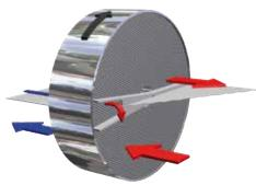
The aluminium rotary heat exchanger with low pressure drop and a temperature efficiency of 80%. The rotor control comprises a step motor with motor control.
