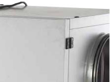
The cabinets are made of Aluzinc AZ185 class C4 according to EN/ISO 12 944-2 and insulated with 50 mm mineral wool. This results in a low noise level to the surroundings/setup room. The panel construction minimizes the formation of thermal bridges in the unit.
