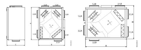
Dimensional drawings for VEX100H = horizontal version and VEX100V- vertical version respectively – both shown with round ducts.
