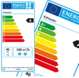
An energy label that states the energy class of the air handling unit in relation to defined operating conditions is available via our product calculation programs.
