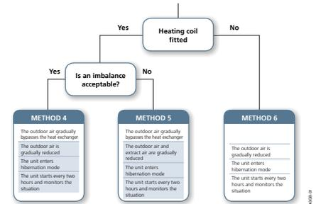
These steps only occur if the effect of the after heating coil is insufficient.
