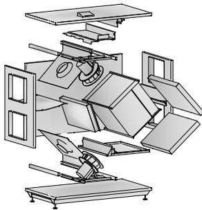
With some projects, limited space means that internal transport of the air handling unit is difficult or impossible. This is why the VEX100CF is available as a split version. It means that the air handling unit can be assembled and tested at the factory as normal – just without sealant. The air handling unit can therefore be easily taken apart at the installation site, transported as single sections, assembled, sealed and commissioned.
