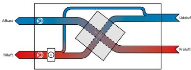
The VEX100CF is designed with a de-icing bypass. If there is a risk of icing, then a certain amount of outdoor air will bypass the heat exchanger and go directly to the after heating coil. This increases the demands on the heating coil's output. However, it avoids a costly preheating coil. The drawing below is an example of a de-icing situation, where 20% of outdoor air is directed through the bypass damper.
