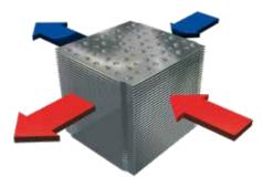
Cross-flow heat exchanger in aluminium with moderate pressure drop and high temperature efficiency. The crossflow heat exchanger ensures full separation of airways, preventing transfer of odours or pollutants to the supply air.
