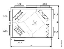
Dimensional drawings for VEX100H = horizontal version and VEX100V- vertical version respectively – both shown with round ducts.
