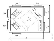
Dimensional drawings for VEX100H = horizontal version and VEX100V- vertical version respectively – both shown with round ducts.
