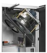
The motor sections are mounted in vibration dampers, which means less noise and vibration in the ducts, and there is no need to install flexible connections between the unit and the duct system.
