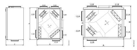
Dimensional drawings for VEX100H = horizontal version and VEX100V- vertical version respectively – both shown with round ducts.
