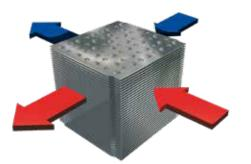
Cross-flow heat exchanger in aluminium with moderate pressure drop and high temperature efficiency. The crossflow heat exchanger ensures full separation of airways, preventing transfer of odours or pollutants to the supply air.
