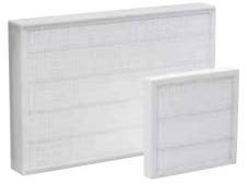
The filter panels are easy to replace and can be ordered as filter class Coarse 85% (M5) or ePM1 55% (F7) according to ISO 16890.
