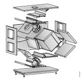
VEX100 IS AVAILABLE AS A SPLIT VERSION. With some projects, limited space means that internal transport of the air handling unit is difficult or impossible. This is why the VEX100 is available as a split version. It means that the air handling unit can be assembled and tested at the factory as normal – just without sealant. The air handling unit can therefore be easily taken apart at the installation site, transported as single sections, assembled, sealed and commissioned.
