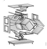
VEX100 IS AVAILABLE AS A SPLIT VERSION. With some projects, limited space means that internal transport of the air handling unit is difficult or impossible. This is why the VEX100 is available as a split version. It means that the air handling unit can be assembled and tested at the factory as normal – just without sealant. The air handling unit can therefore be easily taken apart at the installation site, transported as single sections, assembled, sealed and commissioned.
