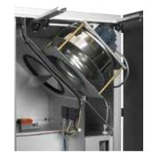
The motor sections are mounted in vibration dampers, which means less noise and vibration in the ducts, and there is no need to install flexible connections between the unit and the duct system. The motor sections are retractable for easier service. The motors are EC type with very high efficiency, meeting the requirements of the EcoDesign directive.
