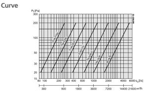
THAV fue gas resistance If the duct system has smoke ventilation, e.g. in apartment buildings, flue gas resistance in the duct system must be calculated from the following diagram. The THFV roof terminal has a fixed flue gas resistance.
