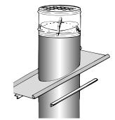
THAV roof terminal is for vertical exhaust and has a built-in damper. A bird protection net is mounted at the top to prevent unwanted objects from entering the duct system.
