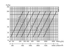
THAV fue gas resistance If the duct system has smoke ventilation, e.g. in apartment buildings, flue gas resistance in the duct system must be calculated from the following diagram. The THFV roof terminal has a fixed flue gas resistance.
