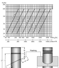
Dimensions E, F and G apply only to PERFORM flashing. With zinc, the flashing is always 100 mm
