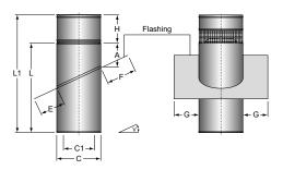
Dimensions E, F and G apply only to PERFORM flashing. With zinc, the flashing is always 100 mm
