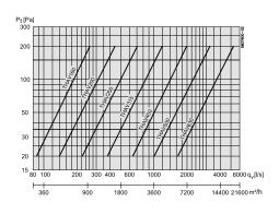
THAV fue gas resistance If the duct system has smoke ventilation, e.g. in apartment buildings, flue gas resistance in the duct system must be calculated from the following diagram. The THFV roof terminal has a fixed flue gas resistance.
