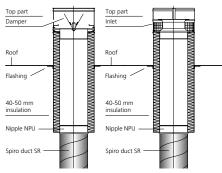
THAV roof terminal is for vertical exhaust and has a built-in damper. A bird protection net is mounted at the top to prevent unwanted objects from entering the duct system.
