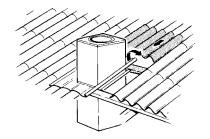
Make a hole in the roof about 30 mm larger than the vent, and loosen overlying tiles/panels, sliding them upwards to permit insertion of flashing.
