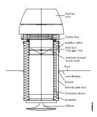
The roof vent has been designed to take an electric cable via the integral cable duct. The installation cable is inserted in the cable duct at the bottom and drawn up by the safety switch, which is not normally an EXHAUSTO delivery. The safety switch is mounted on the control panel as shown in the guide 3004346.
