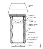
The roof vent is insulated for sound and condensation. To avoid transfer of vibrations to the roof vent, a rubber ring is mounted on the fan.
