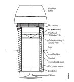
The roof vent is insulated for sound and condensation. To avoid transfer of vibrations to the roof vent, a rubber ring is mounted on the fan.
