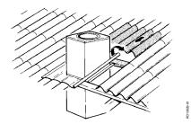
Make a hole in the roof about 30 mm larger than the vent, and loosen overlying tiles/panels, sliding them upwards to permit insertion of flashing.
