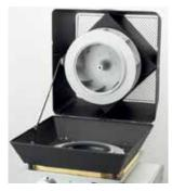
The fan is fitted onto the roof cowl using the supplied vibration dampers, This ensures vibration-free operation, while the mineral wool mat positioned on the spigot forms a seal between the fan and the roof cowl. The safety bolts are fitted in the roof cowl.
