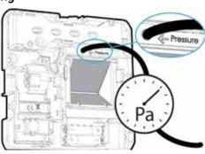
Balancing the valve in relation to desired airflow step  ${\bf 1}\cdot$
