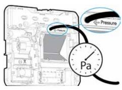
Balancing the valve in relation to desired airflow step
