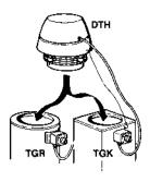
DTH fans are designed for use with TGR or TGK roof cowls, for simple and optimal installation.
