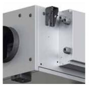
The cabinet is made of 0.8-mm galvanised steel corrosion class C4 in accordance with EN/ISO12944-2and insulated with 50 mm mineral wool. This results in low noise emissions to the surrounding environment.
