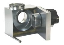
BESF box fans are made from Aluzinc® AZ185 class C4 in accordance with EN/ISO12944-2 and sound and condensation-insulated with 30 mm mineral wool.
