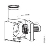
To minimise system pressure drop when connecting to a duct system, we recommend the use of an OGSR transition piece (accessory).
