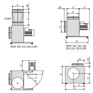
The BESF box fan can be mounted in various positions. Note, however, that the ventilator must not be positioned with the motor turned downwards.
