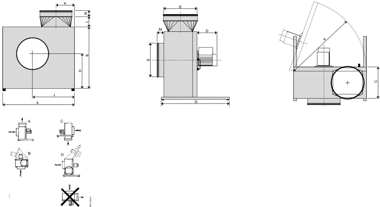
The box fan can be mounted in different positions, however, space for insulating the ducts must be taken into account.
