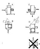
The box fan can be mounted in different positions, however, space for insulating the ducts must be taken into account.
