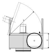
The box fan can be mounted in different positions, however, space for insulating the ducts must be taken into account.
