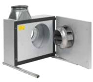
BESB box fans are made from Aluzinc® AZ185 class C4 in accordance with EN/ISO12944-2 and insulated with 50-mm mineral wool.
