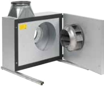
BESB box fans are made from Aluzinc® AZ185 class C4 in accordance with EN/ISO12944-2 and insulated with 50-mm mineral wool.
