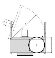
The box fan can be mounted in different positions, however, space for insulating the ducts must be taken into account.
