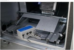
• Remove the four bolts at the front of the rail system.
