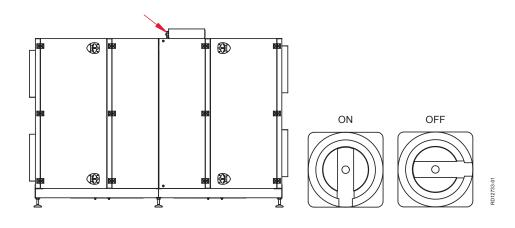
Lock the air handling unit during operation
