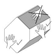
The counter flow heat exchanger can be removed from both sides of the unit. Choosing the side that is opposite the connection box on top of the unit avoids having to remove the bypass damper.
