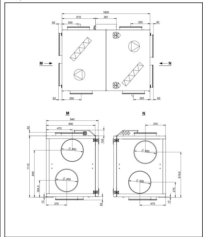
NB The drawing shows all of the spigot positioning options. Spigot positioning marked with \* is not available for VEX units with a bag filter.
