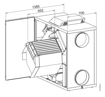
**NB:** For servicing, the VEX must have a free height of at least 300 mm above the connection box.
