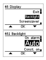
Use the ▲ and ▼ buttons to navigate through the menu to **Backlight** and press the **OK** button.
