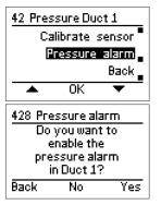
The pressure tolerance can then be set in the range 0 - ±500 Pascals pressure with a factory setting of ±100 Pascal.
