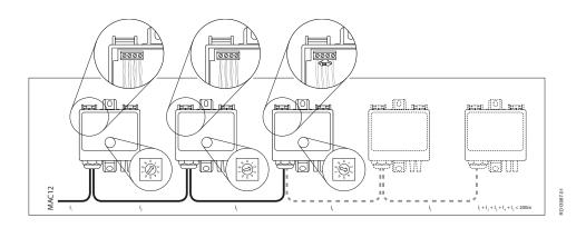
When MAC12 is set up to regulate multiple ducts, the individual pressure sensors must be adjusted so that the control system can read them.
