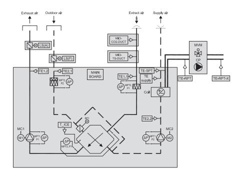
The simplified diagram shows a VEX unit with RIGHT fan placement. See table of designations on next page.
