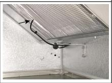
Check that the sensor  $T_{ice}$  is correctly positioned. The sensor must protrude approx. 10 mm between the heat exchanger fins, as otherwise the sensor will not measure correctly.
