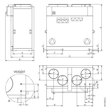
The indicated dimensions **A-P** are shown on the dimensional drawing and can be read off from the tables next to the given VEX size.
